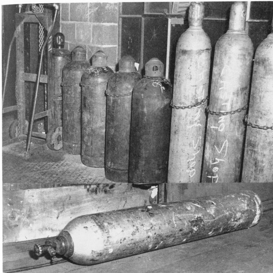
Upper photo:—The Casting Shop provides safe storage for cylinders. They are capped, chained to a wall in an area where fire is most unlikely. At the left may be seen a special hand truck for transporting them safely.
